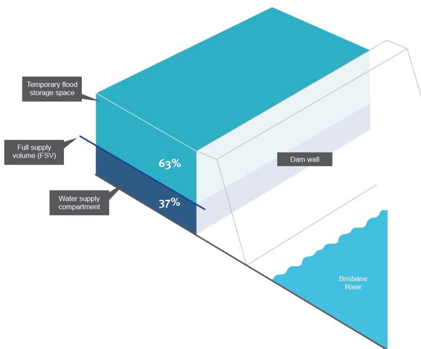
It is important to remember that Wivenhoe and Somerset dams, as flood mitigation dams, are not near their total capacities when their water supply storage compartments are full. Both dams have much more space specially reserved for dealing with floodwaters. For Wivenhoe Dam, the water supply storage compartment can hold up to 1.165 million megalitres of our drinking water, which is less than 40 per cent of the total 3 million megalitres capacity of the dam.
