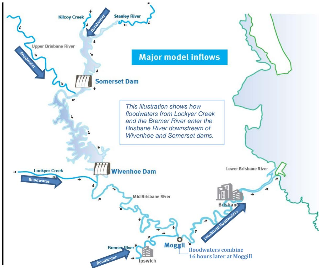
The dam operators measure the floodwaters in the Brisbane River at Moggill as it is the first place where major floodwaters all combine. The dam operators try to avoid the highest releases from Wivenhoe Dam arriving at Moggill at the same time as the highest floodwaters from Lockyer Creek and the Bremer River.
